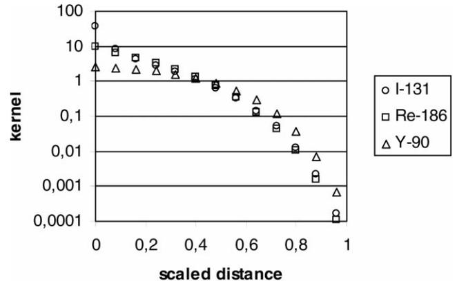
Fig. 1. Beta dose point kernels of  $^{131}\text{I}$ ,  $^{186}\text{Re}$  and  $^{90}\text{Y}$ . The radial distance is scaled by the range of the isotope.
