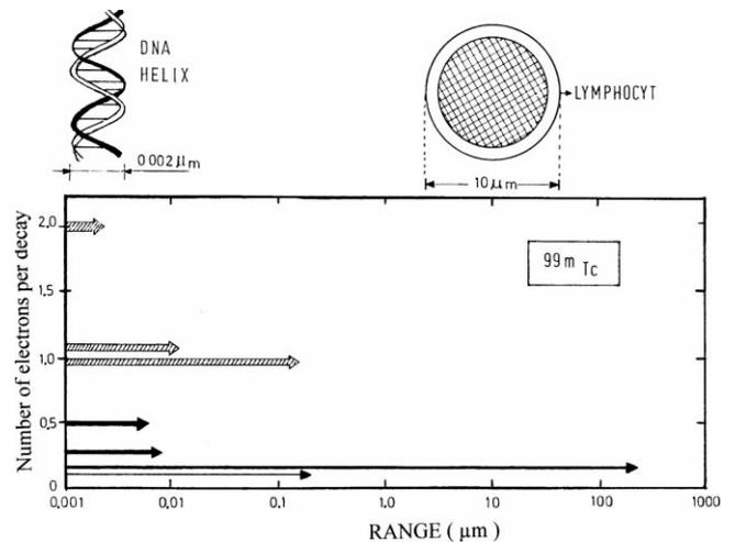
Fig. 6. Comparison of the range in tissue for the important low-energy Auger electron groups in the decay of  $^{99m}\text{Tc}$  with the dimensions of a lymphocyte and the DNA double helix structure.
